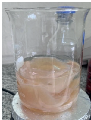
Figure 1 - BNC membrane after the purification process.
