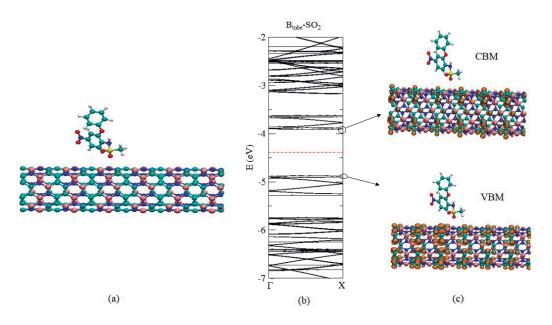
Figure 8 - Geometry of equilibrium (a), electronic band structure (b) and LDOS associated to VBM and CBM for  $B_{hube}$ -SO<sub>2</sub>.
