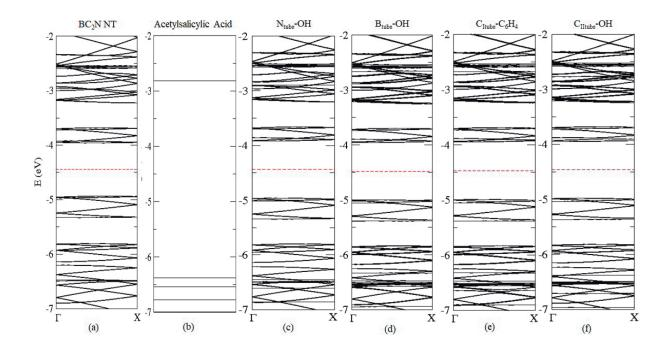
In figures 6 and 7 it is observed little or no significant change around the Fermi energy in the electronic band structures indicating a weak interaction between BC2N NT and molecules, which is in agreement with the values found for binding energies. In figures 8 and 9 we can observe the relaxed
