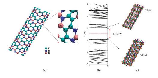
$BC_2N$  nanotube (3,3) has a diameter of 8.34 Å and 48 atoms in its unit cell. The bond lengths of the C-C, B-N, C-N and C-B were found to be on average, 1.44 Å, 1.44 Å, 1.39 Å and 1.54 Å, respectively, which is in agreement with the literature (MIYAMOTO et al., 1994).
