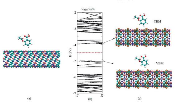
Figure 9 - Geometry of equilibrium (a), electronic band structure (b) and LDOS associated to VBM and CBM for  $C_{ltube}$ - $C_{6}H_{4}$ .
