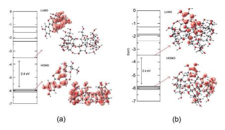
Furthermore, the plots of electronic charge density for the LUMO (Figure 3 (a)) show a contribution on the mangiferin and a distribution in the HOMO for the mangiferin molecule as well as beta-CD. From the Mulliken population analysis, the charge transfer systems studied show that the CD behaves as an electron acceptor for mangiferin interacting on outer configurations of beta-CD. Based on the binding energy results for mangiferin adsorbed on the outer surface of the beta-CD
